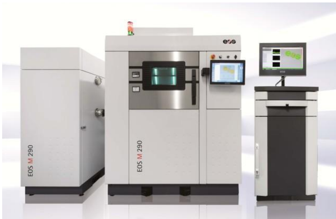
Figure 4: Laser powder bed fusion system used for metal AM training and development.
