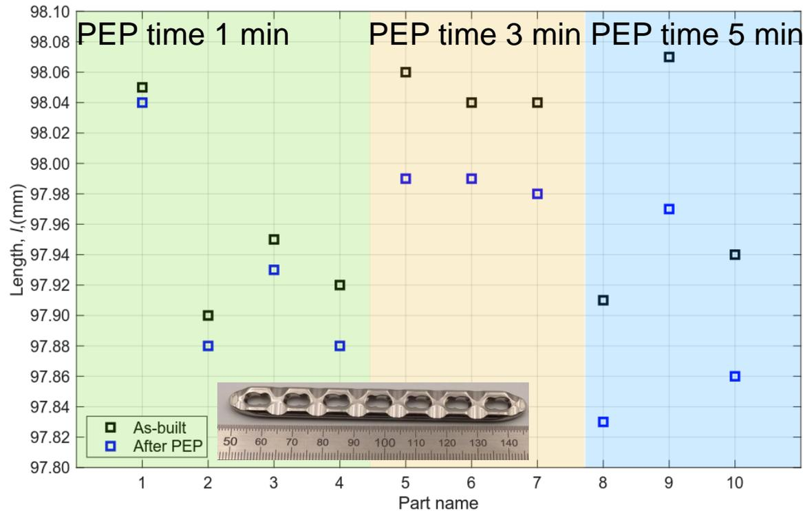
A length of titanium parts before and after the PEP process.
