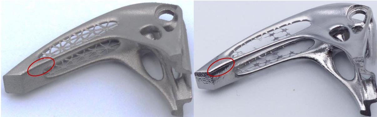
Additively manufactured parts out of Ti6Al4V before (left) and after (right)
