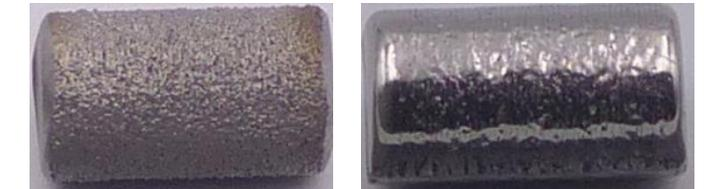
Additively manufactured parts out of CrMnNi before (left) and after (right) PEP
