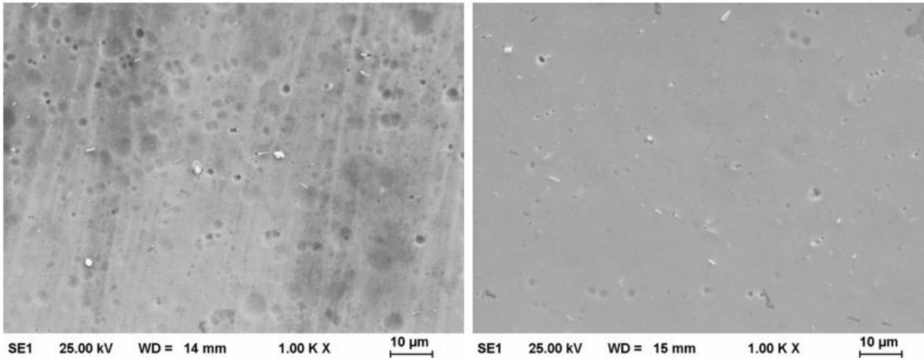
SEM pictures of Nitinol plates before (left) and after (right) PEP. The process time 3 min
