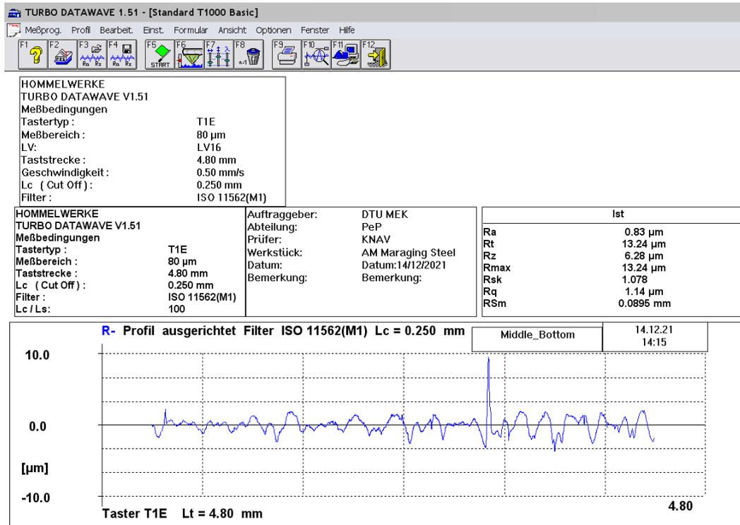
Measurement protocol of a tactile profilometer *TURB.*
