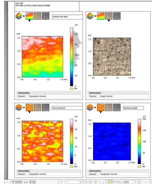
A segment of a measurement protocol of a 3D-profilometer *Mahr.*
