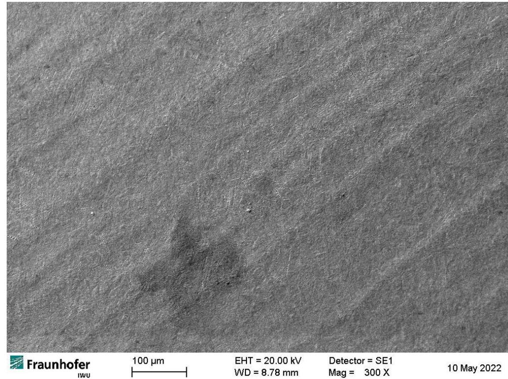
SEM pictures of carburised steel gear segment before (left) and after (right) an additional PEP step. The additional PEP process time 6 min
