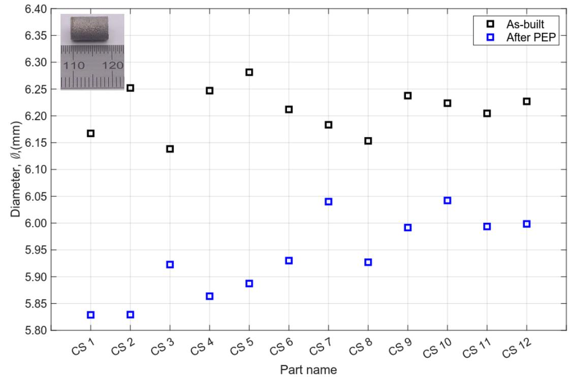
A diameter of austenitic steel parts before and after the PEP process. PEP duration was 30 min.
