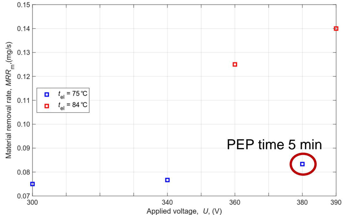
$MRR_m$  of additively manufactured AMZ4 as a function of applied voltage. PEP time 10 minutes.
