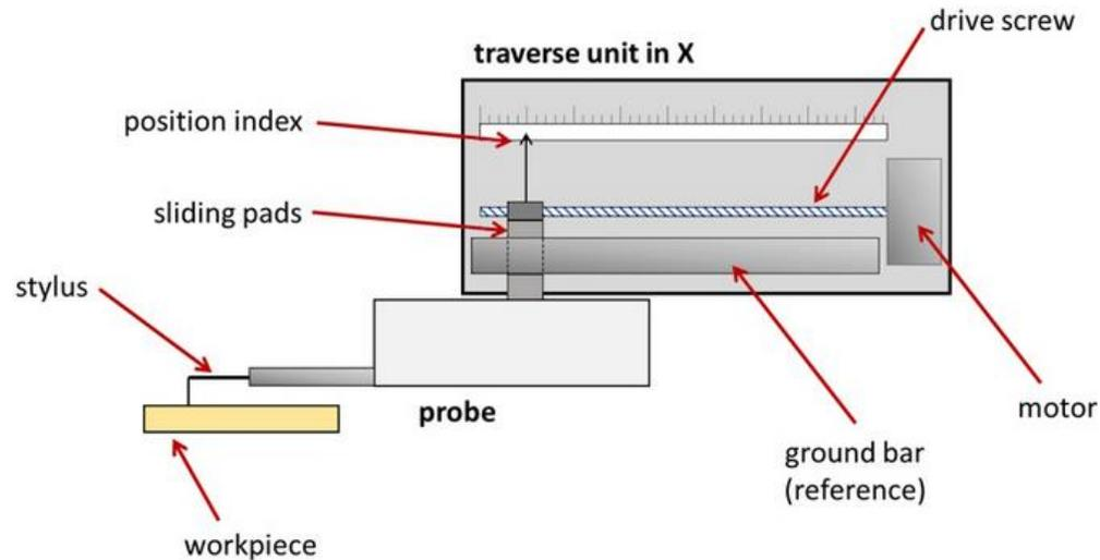
Working principle of a stylus profilometer
