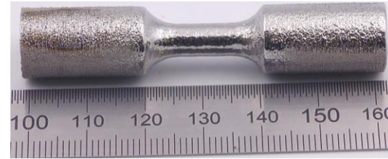
After standing-wave-PEP. Rotation angle was \theta = 120^\circ
