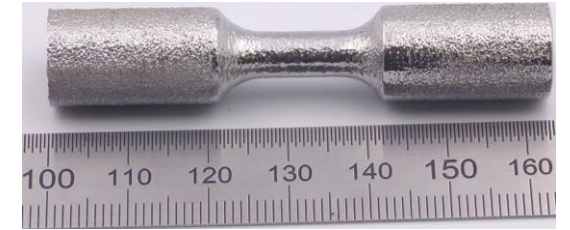
After standing-wave-PEP. Rotation angle was \theta = 90^\circ
