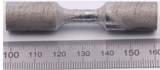
After standing-wave-PEP. Rotation angle was \theta = 180^\circ
