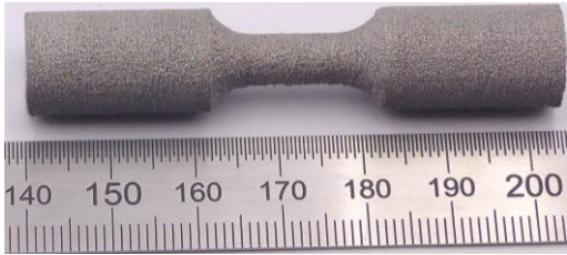
Austenitic steel part in as-built condition
