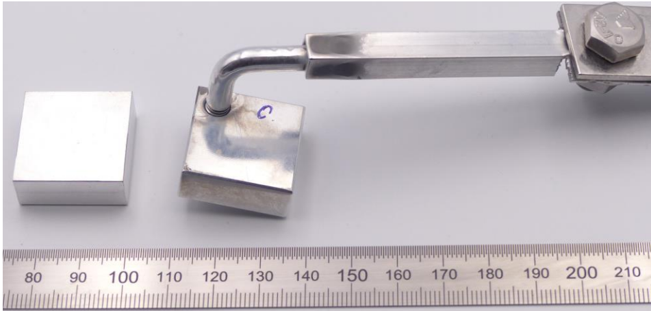
An aluminium holder for aluminium cubes.
